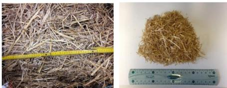
Milling process was applied, increasing the surface area and accessibility of the enzymes to substrate, increasing the saccharification rates and yields.
